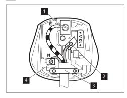
The wire coloured green and yellow must be connected to the terminal marked with the letter «E» or by the earth symbol  $\stackrel{\bot}{=}$  or coloured green and yellow.
